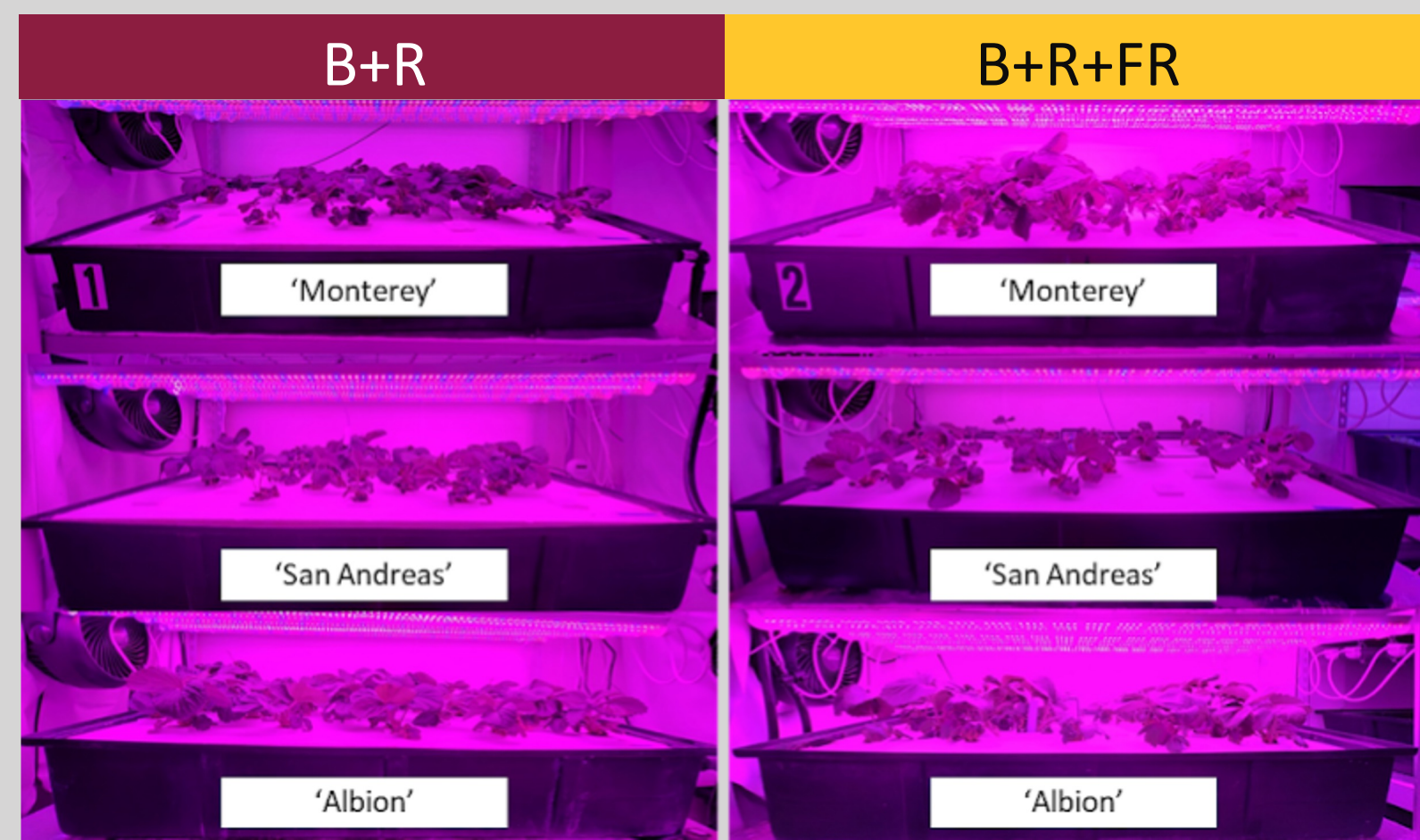
Fig 2. Experimental set up for blue+red (B+R) (left) or blue+red+far-red (B+R+FR) (right) lighting treatment delivered from LEDs.
